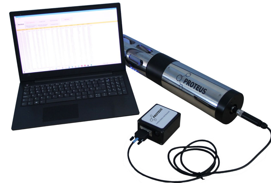
Figure 38: Proteus connected via BBP to a Bluetooth enabled laptop.
