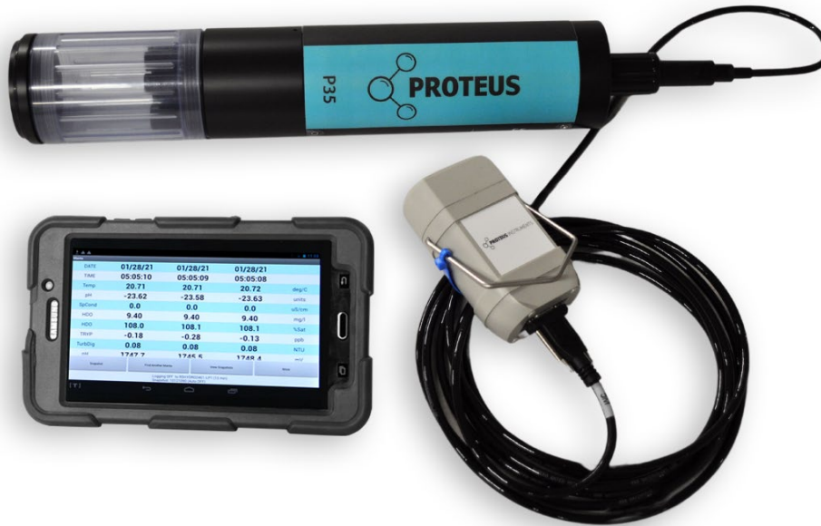
Figure 53: Proteus connected via BBP to a Bluetooth enabled tablet.
