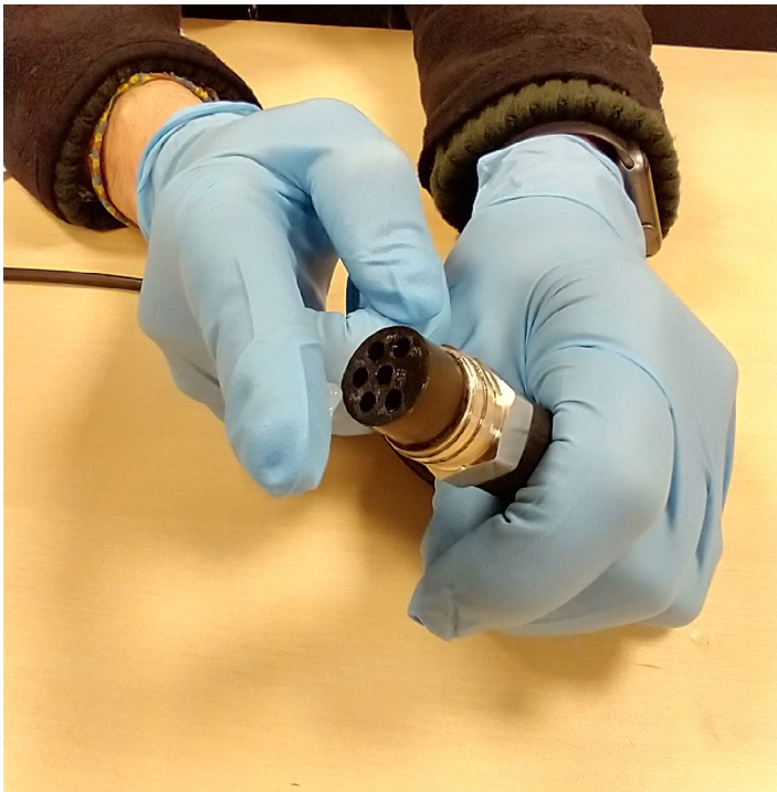
Figure 20: Applying Molikote 111 to the connector plug
