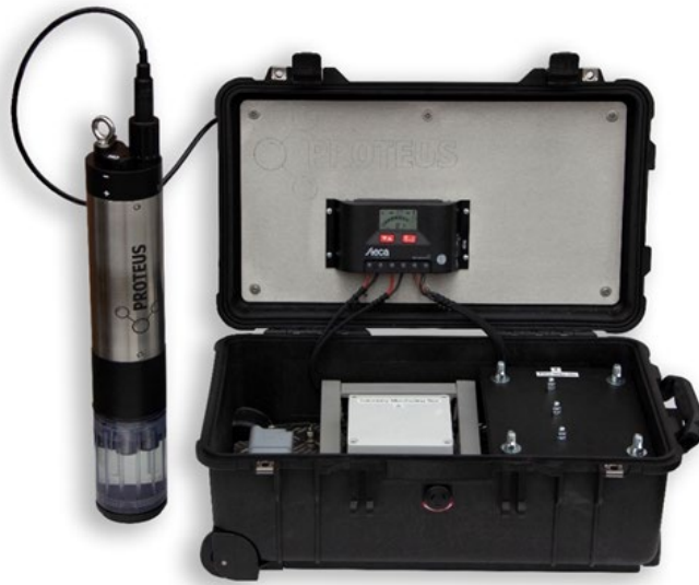
Figure 7: An example of a Proteus set-up using solar power and transmitting data via to the outpost cloud server.
