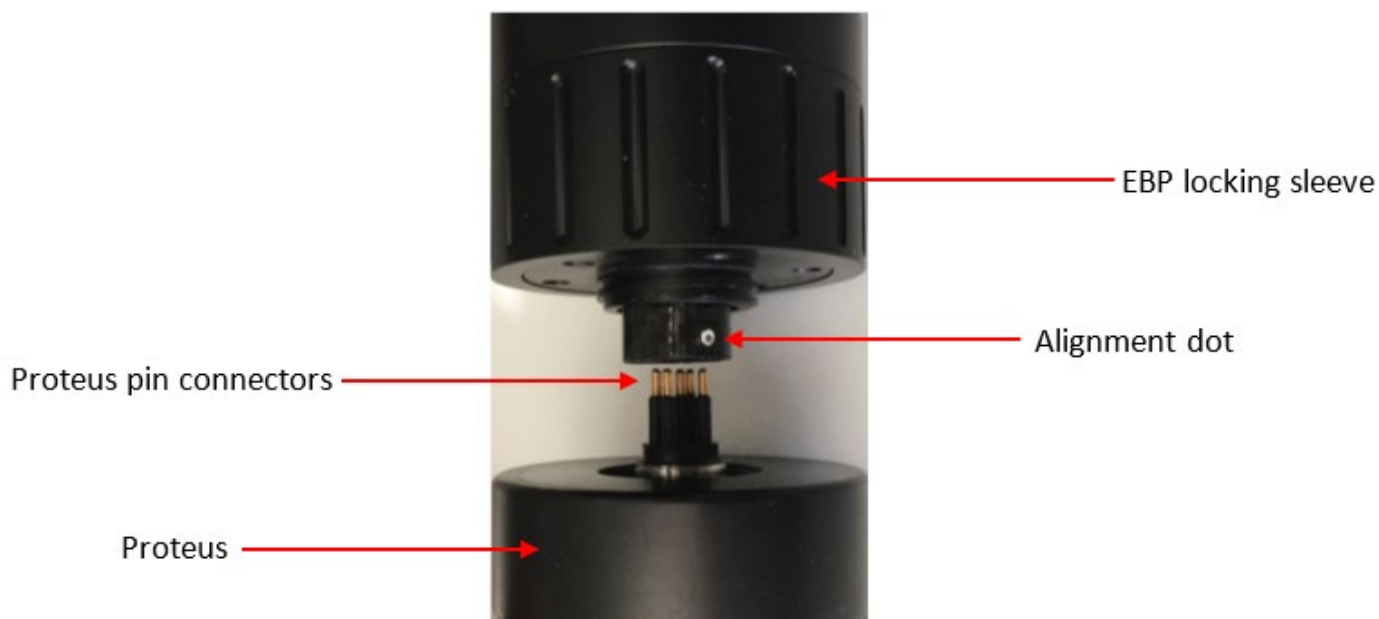
Figure 37: Connection of an EBP to a Proteus probe.
