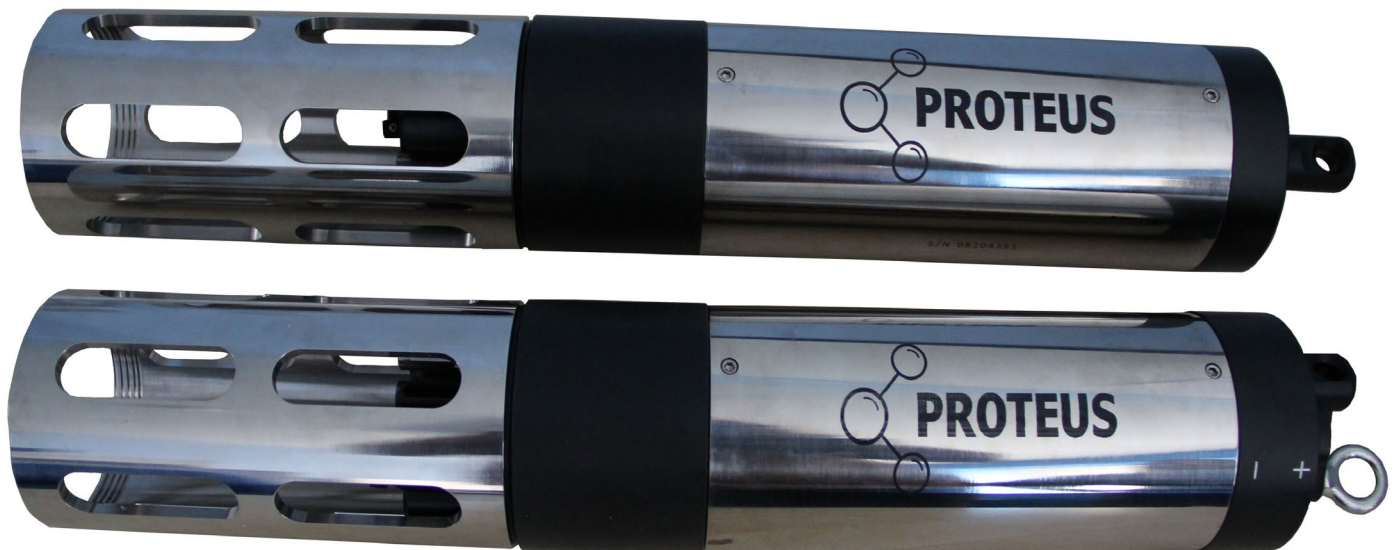
Figure 6: Direct comparison of Proteus with IBP (foreground) and Proteus without IBP (Background).
