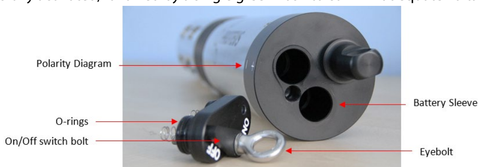
Figure 36: Changing of IBP batteries
