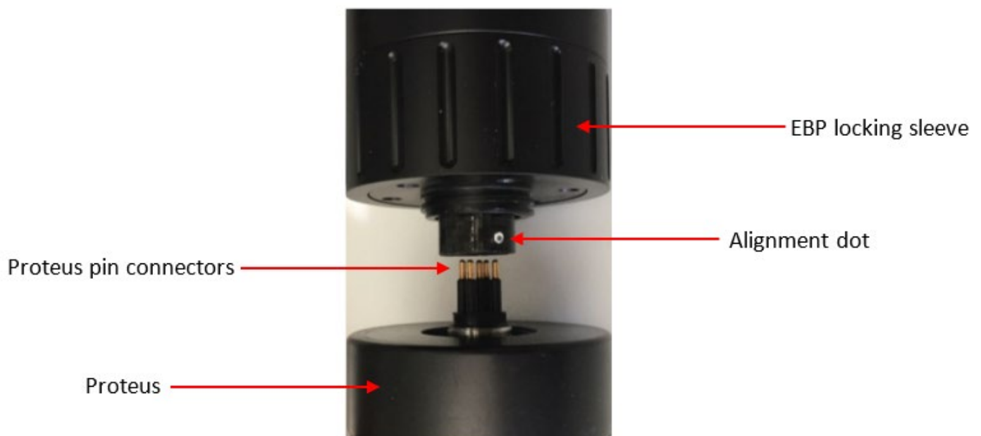
Figure 33: Connection of an EBP to a Proteus probe.
